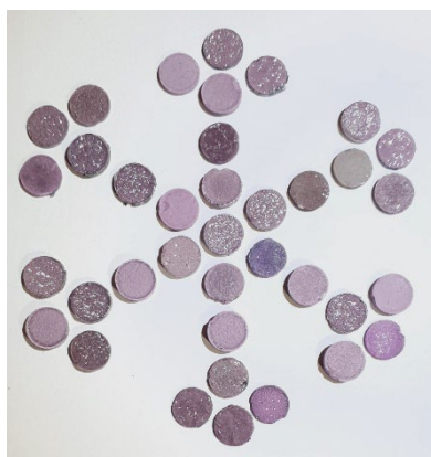
Figure: Pellets of molecular compounds for barocaloric refrigeration.
